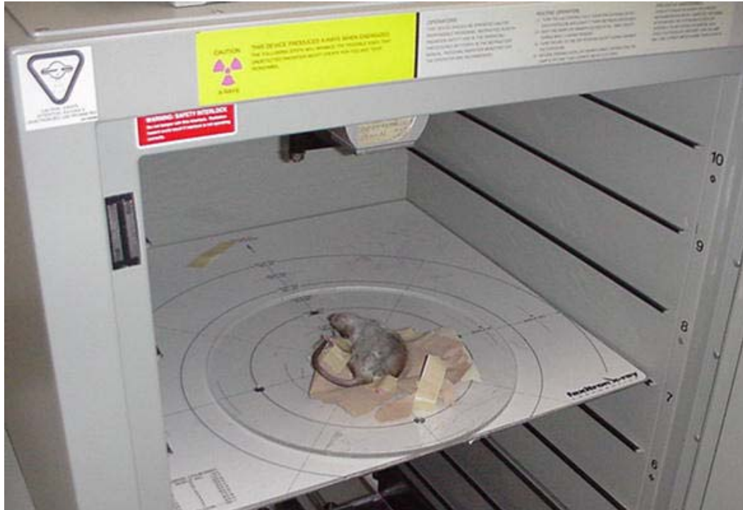
Figure 1 Interior of Faxitron cabinet. An anesthetised rat is placed on a tray mounted at shelf position 7. The x-ray tube can be seen at the top.
